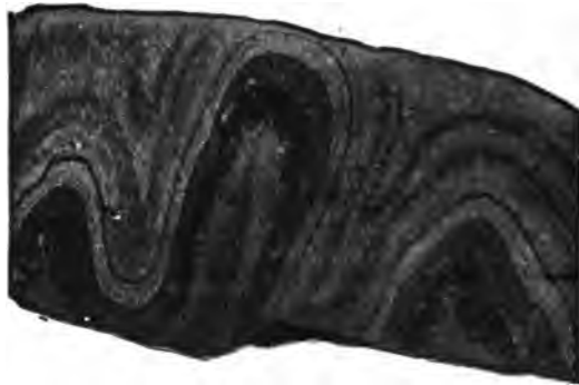
Fig. 196.—Strongly wrinkled portion of the blende layer with dark bands of gray gneiss. (One-half natural size.)
