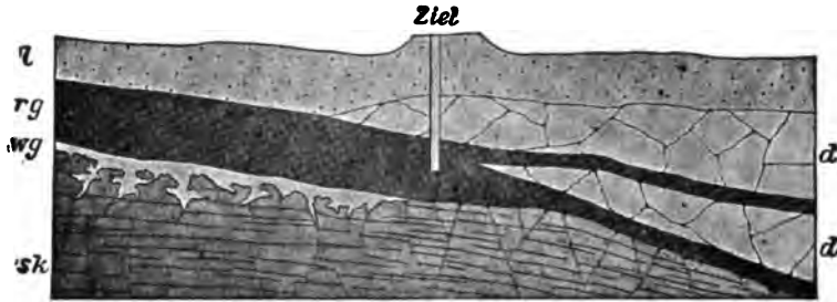
Fig. 229.—Section through the Judith and Scharley mines. (F. Römer.) l, clay; d, dolomite; sk, basal limestone; wg, white cadmia; rg, red cadmia.
