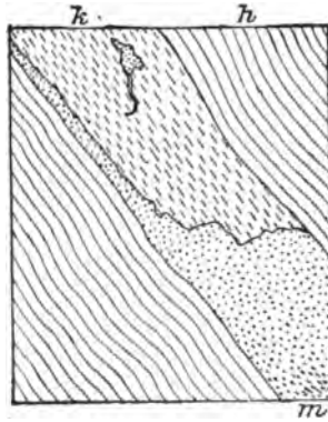
Fig. 241.—Section of the Mutter Gottes bed of Berggiesshübel. h, hornblende schist; n, actinolite; k, crystalline limestone in magnetite.
