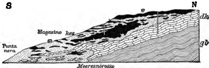
Fig. 245.—Section through the iron ore deposits of Calamita. (Fabri.) dk, crystalline dolomite; e, iron ore; kes, lime-iron-silicate rock.
