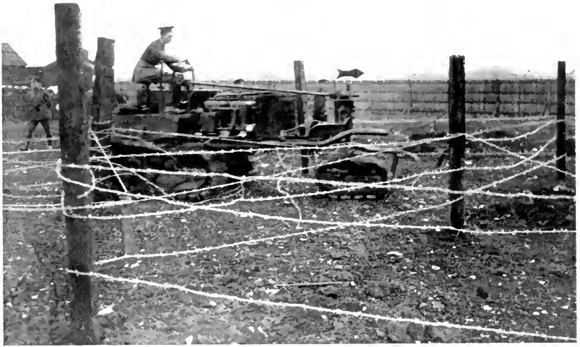
Killen-Strait Machine fitted with Wire Cutting Apparatus. (f 26)
