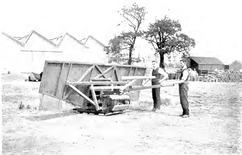
Pedrail Hand Machine fitted with Infantry Shield. (p. 24)
