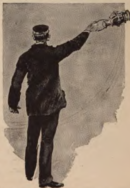
A lamp swung vertically in a circle at arm's length across the track, when the train is running, is the signal that the train has parted.
