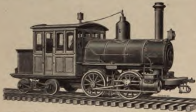
Fig. 32.—"Forney" Tank Locomotive. By the Rogers Locomotive and Machine Works, Paterson, N. J.
