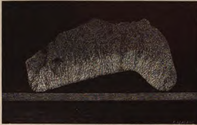
Fig. 52.—Section of the Tread and Flange of a Car Wheel.
